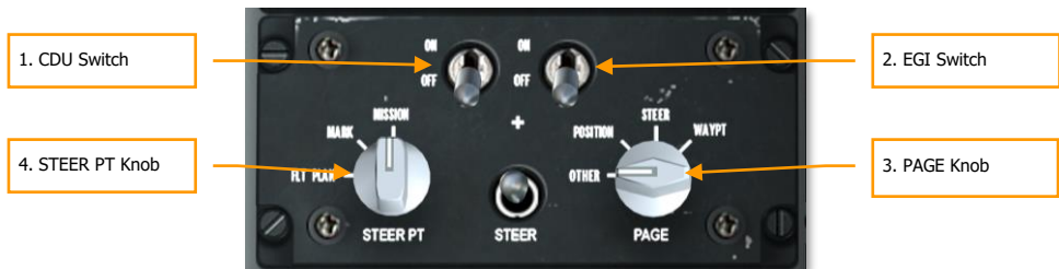
Figure 306. Auxiliary Avionics Panel
