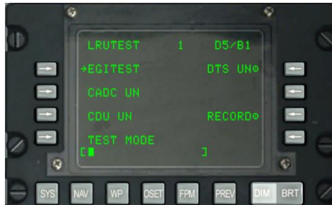
Figure 171. System / LRU Test Sub-Page
