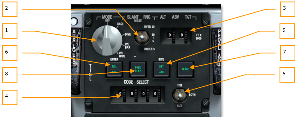
Figure 91. TISL Control Panel
