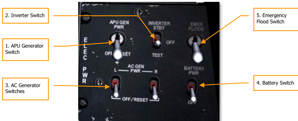
Figure 303. Electrical Power Control Panel
