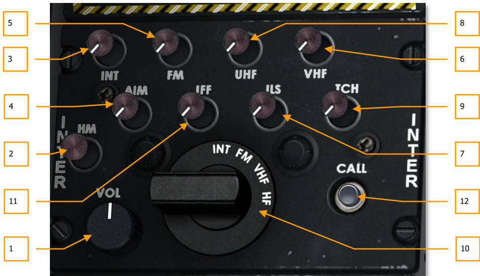
Figure 120. Intercom Control Panel
