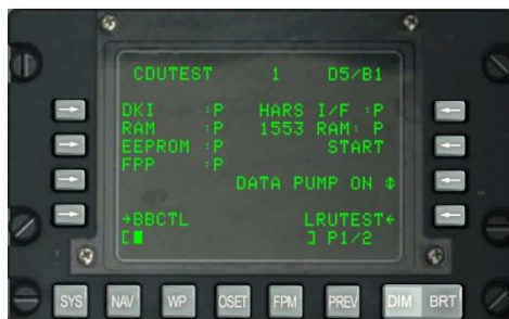
Figure 176. System / CDU Test Sub-Page 1
