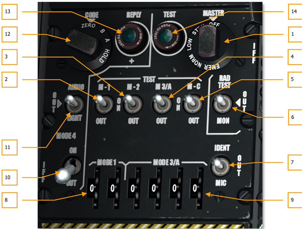
Figure 118. IFF/SIF Control Panel
