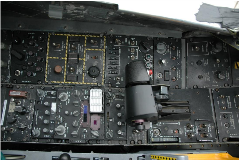
Figure 38. Left Console Showing VHF and UHF Radios
