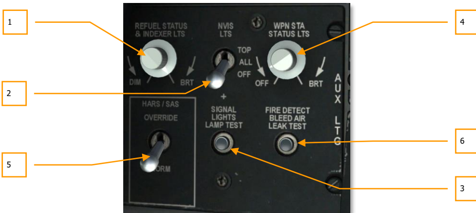
Figure 116. Auxiliary Lighting Control Panel
