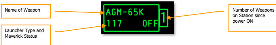
Figure 455. Maverick Station Box Loading, Power Off
