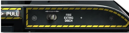
Figure 93. Fire Extinguisher Discharge
