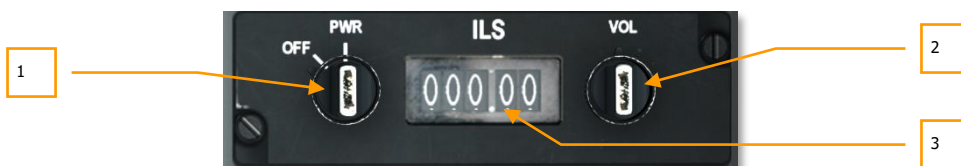
Figure 129. ILS Control Panel
