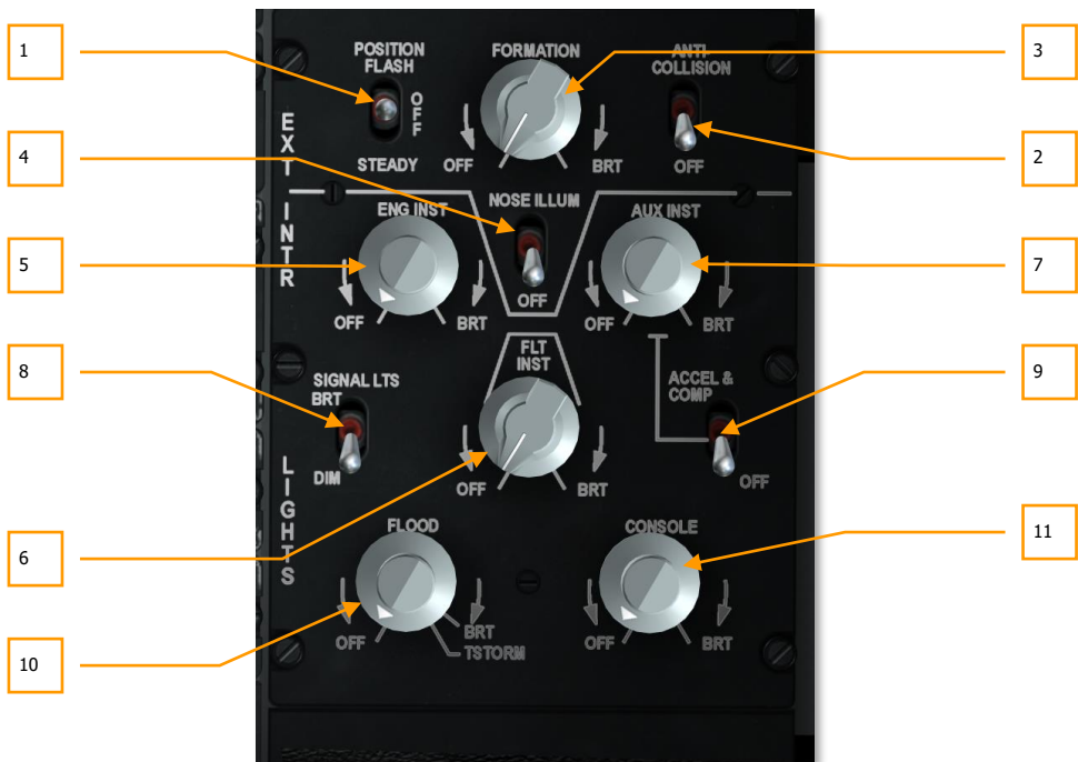
Figure 126. Light Control Panel
