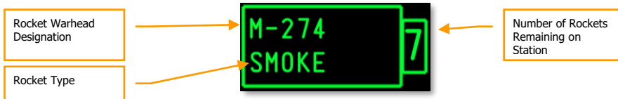
Figure 408. Rocket Loaded Station
