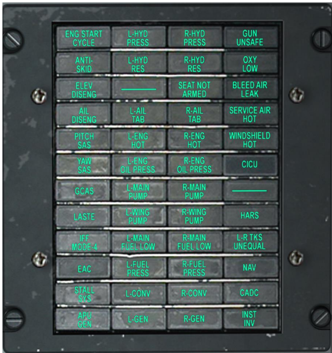
Figure 127. Caution Light Panel
