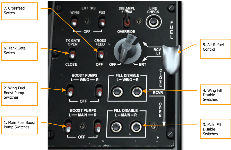
Figure 298. Fuel System Panel
