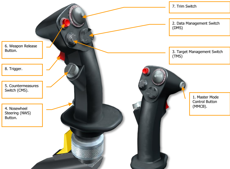
Figure 69. Control Stick
