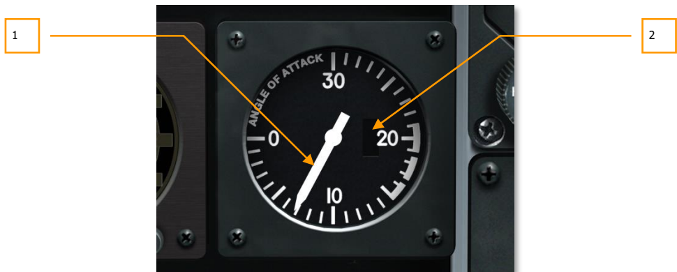
Figure 77. Angle of Attack Indicator
