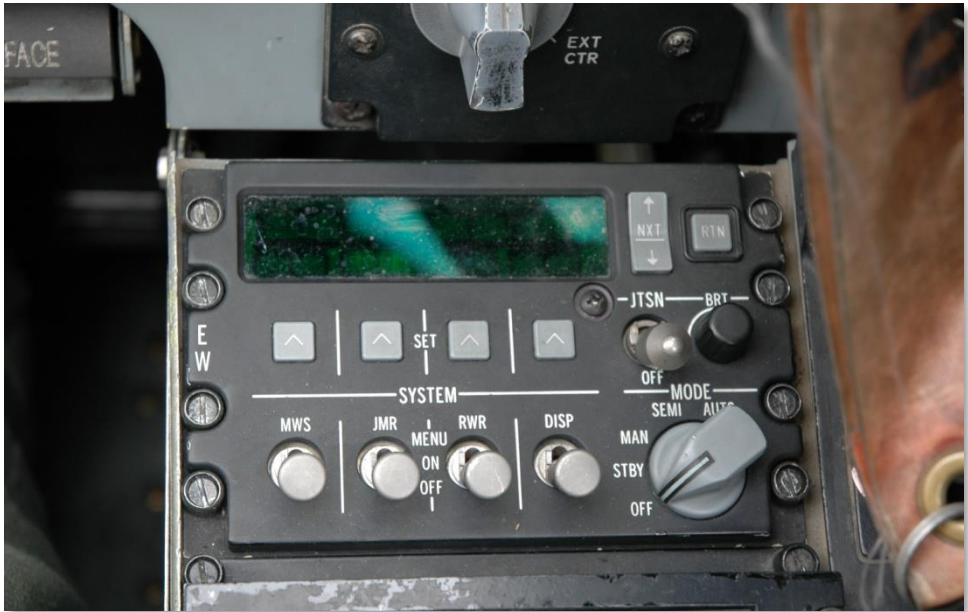
Figure 39. Countermeasure Signal Processor (CMSP) Panel
